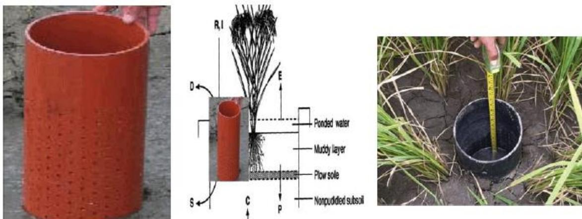
Fig. 6.4: A simple perforated pipe (water tube) installed in the rice field allows farmer to monitor water level beneath the soil surface (Kulkarni, 2011)
