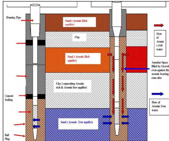
Fig.6.3: Tube-well design of a deep tube well tapping safe deeper aquifer
